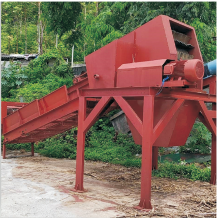
图 10 甘蔗除杂机断尾试验装置 Fig. 10 Tail-breaking test device of sugarcane impurity remover
