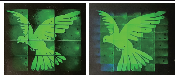
图20 重叠打印前后两张全息图的再现图像对比 Fig. 20 Comparison of the reconstructed images of two holograms without and with overlapped printing
