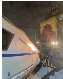
e 采用内燃机车救援着火动车组 e EMU rescue by diesel locomotive rescue station
