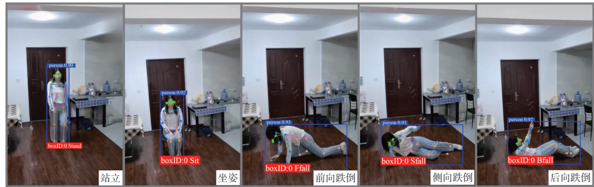
图 11 硬件终端姿态识别效果图 Fig. 11 Diagram of hardware terminal pose recognition effect
