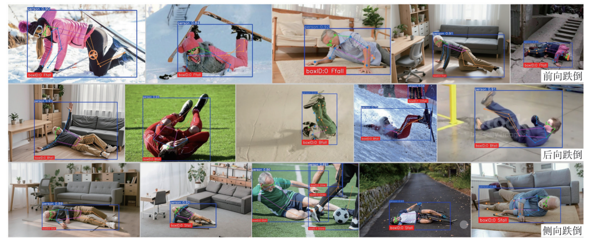
图9 跌倒方向判别效果图 Fig. 9 Diagram of fall direction discrimination result
