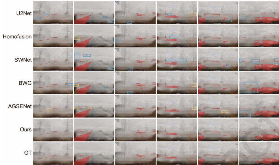
Fig. 8. Representative prediction results on the Foggy-Puddle dataset, comparing ABCDWaveNet (ours), AGSENet, BWG, SWNet, Homofusion, and U2Net. The bottom row shows the ground-truth annotations. Yellow boxes denote missed detections, while blue boxes indicate false detections.
