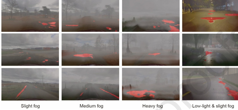
Fig. 10. ABCDWaveNet detection results across varying fog densities and road types, including slight fog, medium fog, heavy fog, and low-light & slight fog, demonstrating the model's robustness and generalization capability under diverse environmental conditions.
