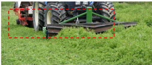
图8 前置人字形罗代尔式碾压机 Fig.8 Front-mounted herringbone Rodale Roller Crimper
