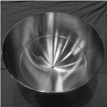
图 13 TC4 钛合金贮箱半球成品样件 Fig. 13 Final hemisphere shell of TC4 titanium alloy storage tank
