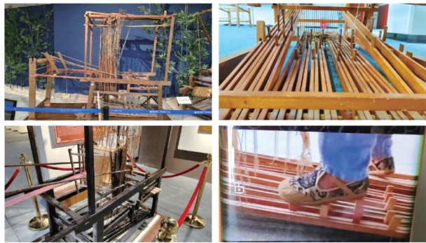
图3 丁桥织机综躡结构细节 Fig. 3 Detailed structure of heddle treadle of the Dingqiao loom
