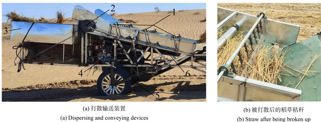
1. 拨草齿; 2. 曲柄; 3. 储料箱; 4. 发动机; 5. 压草碾轮; 6. 钉齿输送带 1. Toothing; 2. Crank; 3. Hopper; 4. Engine; 5. Grass roller; 6. Spike conveyor belt
