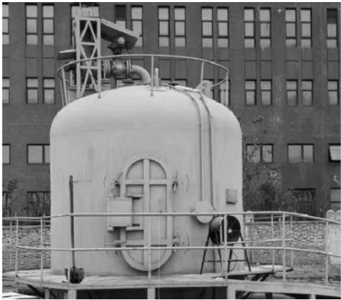
图 1 爆炸碉堡实物图 Fig. 1 Physical view of the exploding bunker
