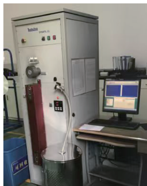
图 1 试验所用 DYNAFIL CU 动态热应力仪实物照片 Fig. 1 Photograph of DYNAFIL CU dynamic thermal stress tester used in experiment
