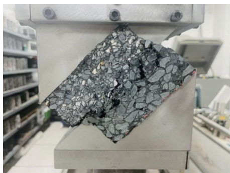
(b)OGFC-16+OGFC-10 黏结层破坏
