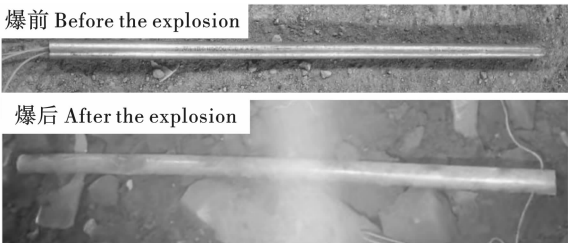
图 17 无钢制切缝聚能管的爆破结果 Fig. 17 Blasting results without steel slitted shaped charge tube
