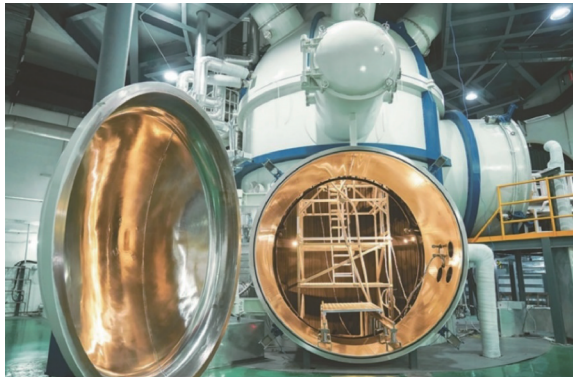
图5 空间环境地面模拟装置系统级综合辐照舱 [28] Figure 5 The comprehensive irradiation facility of the SESRI [28]
