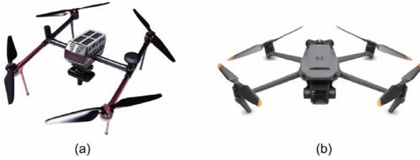
Fig. 8. Two models of UAVs used for collecting point clouds of the investigated large cable-stayed bridge. (a) Feima D2000S; (b) DJI Mavic 3E.
