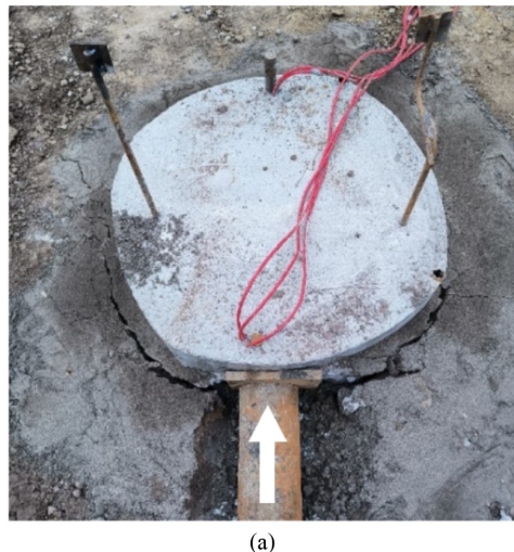
Fig. 14 Failure modes of RP2 pile and surrounding ground under individual horizontal load: (a) on-site failure situation of ground surface; (b) schematic of short pile-soil-inclined anchor interaction.
