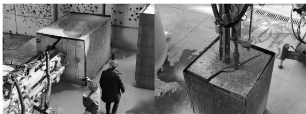
图6 钢模板拆除前混凝土试件破裂样貌 Fig. 6 Cracked appearance of concrete specimens before removal of steel formwork
