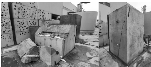
图7 钢模板拆除后混凝土试件破裂样貌 Fig. 7 Cracked appearance of concrete specimens before removal of steel formwork
